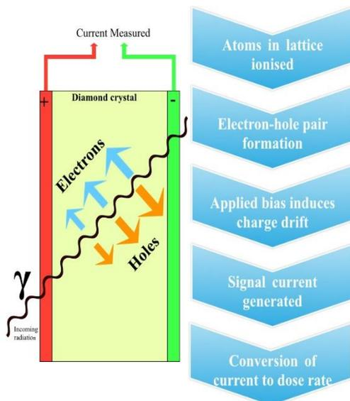
Principle of dose rate measurement in diamond detectors
