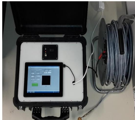
Portable dose rate measurement hardware and software
