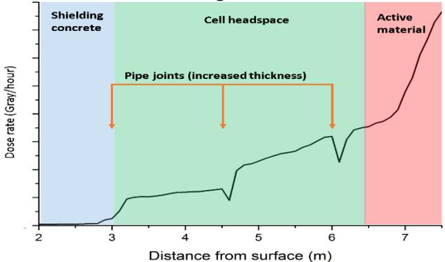
Detector response with distance from surface recorded in an active cell at the Sellafield site.
