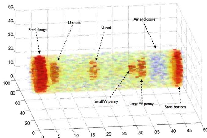
Reconstructed objects encased in a concrete waste drum.
