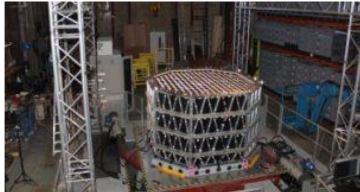
Fig 1: physical model of AGR on the seismic testing table
