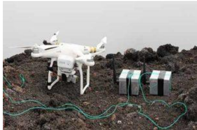
The sensor units with UAV ready for deployment
