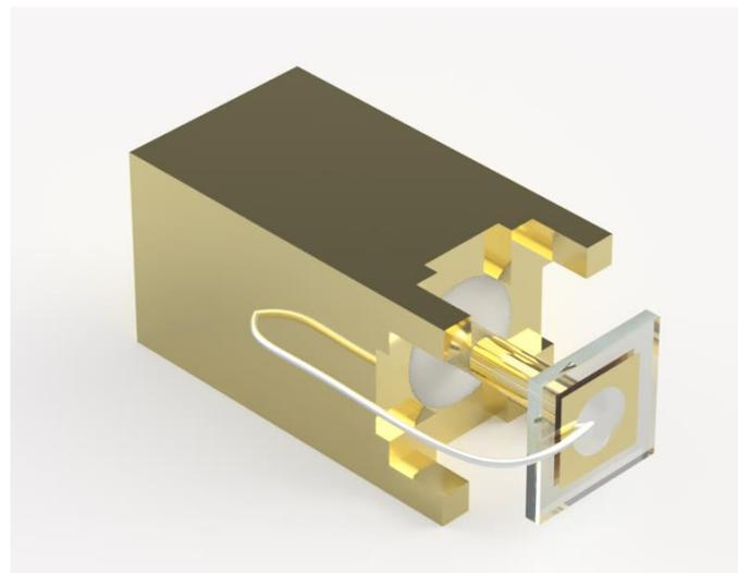
**Figure 1:** A render of the as-constructed diamond gammavoltaic, mounted on an SMA head for testing, and here reproduced for monte carlo simulation purposes.
